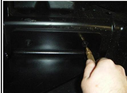
4. Lower hitch and drill (4) 17/32" holes marked in Step (3).
