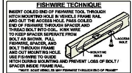
6. Reverse fishwire (2) 1/2-13 x 1 3/4" carriage bolts and SP6 spacers into the access holes.
