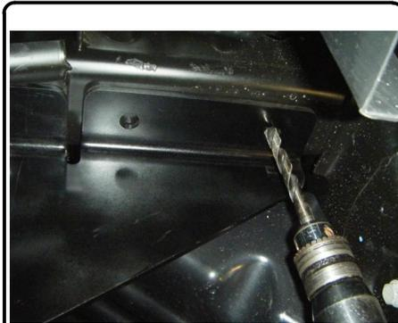
5. Fishwire (4) 1/2-13 x 1 3/4" carriage bolts and SP6 spacers through the access holes and out drilled holes.
