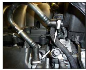
3. Depress the locking tabs and then disconnect the crank case vent line from the intake plenum and valve cover vent port.
