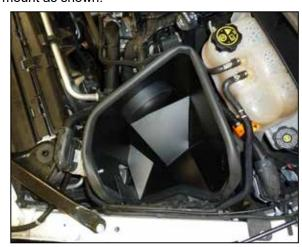
14. Install the heat shield assembly into the vehicle so the mounting grommet slides into the factory mounting hole. Slide the fresh air intake scoop into the opening in the heat shield and resecure to the core support with the factory clip. Secure the heat shield with the factory nut removed in step #9.
