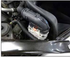
15. Connect the wiring bulk connector onto the bracket installed onto the heat shield.
