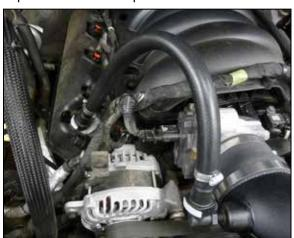
24. Connect the crank case vent hose assembly to the valve cover port and then to the fitting installed into the intoler tube.
