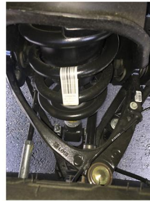
One Piece Cast Upper Control Arm
