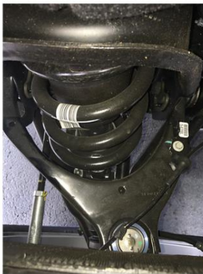
Two Piece Stamped Upper Control Arm
