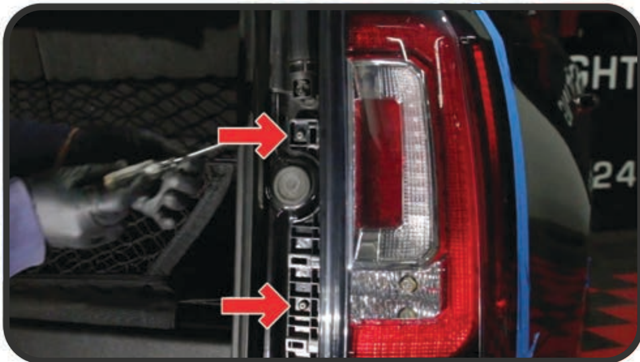
STEP 4: REMOVE TWO T15 TORX BOLTS
