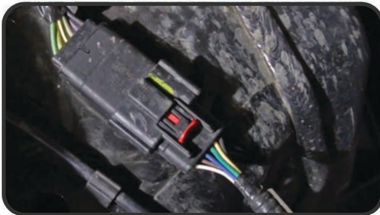
STEP 5: LAY ON THE FLOOR, LOOK FOR THE TAIL LIGHT HARNESS
