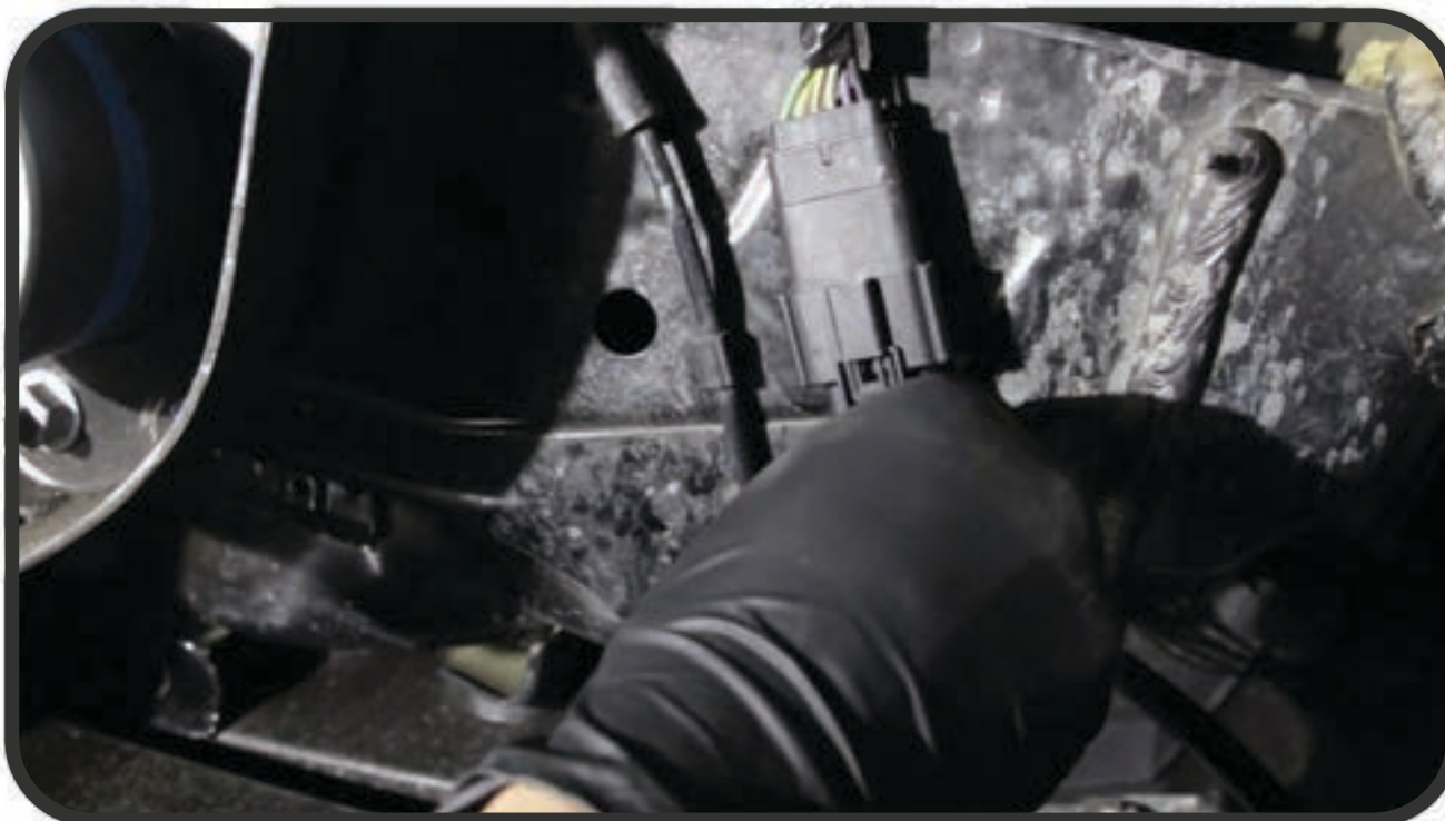
STEP 15: GO UNDER THE CAR AND PLUG IN THE HARNESS
