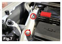
8. Remove the following Torx T-15 screws from the front passenger side fender liner.
