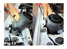
12. Align the mounting bracket bolt holes with the radiator support bracket and battery tray, then tighten the bolts. Once secured, place the lid back on the catch can. (Fig.14).
