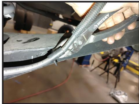
**12.** Install the remote reservoir now using the supplied bracket, hose clamp and self-tapping 3/8 bolt and 3/8 split locker washer. Hold the reservoir and bracket up to position and mark the hole for drilling with the 11/32 drill bit. Once drilled, install the bracket with hose clamps installed, then attach the reservoir. (Some models may have an exhaust on the driver side. The reservoir will need to be mounted a little higher on the frame to clear.) [FIGURE 12 & 13]
