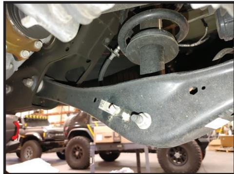
**8.** Grab the ICON coilover assembly now and install the upper mount into the coil bucket using the supplied 3/8 bolts, flat washer and split lock washer. The split lock washer goes on the bolt before the flat washer. Torque to 35 ft-lbs. [FIGURE 7 & 8]
