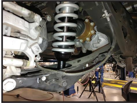
**10.** Reinstall the brake line bracket and lower control arm pivot bolt. Torque the pivot bolt to 180 ft-lbs.
