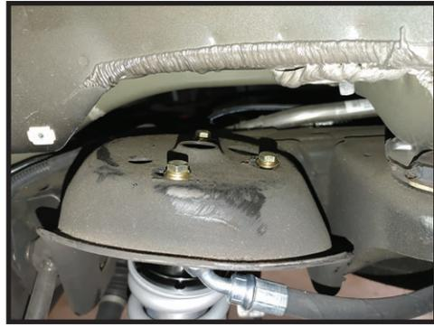
**9.** Install the lower coilover hardware using the OEM bolt and nut. Torque to 100 ft-lbs. [FIGURE 9]
