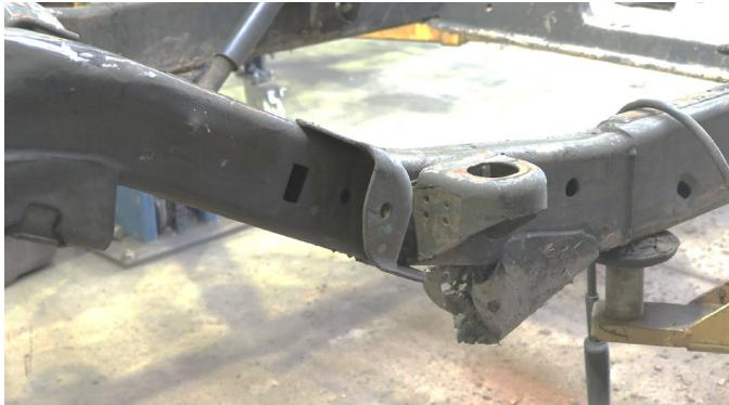
Remove your rear wheel, and disconnect the control arm from the mount.
