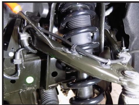
4. Remove the 10mm bolts holding the brake lines and sensor wire onto the knuckle. Also remove the speed sensor itself from the front side of the knuckle, using a T27.
