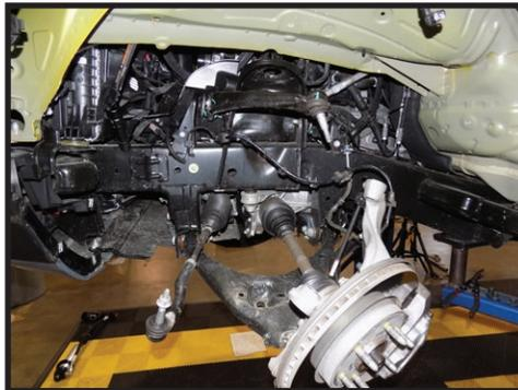
**11.** Using a 21mm ratchet and 21mm wrench, loosen and remove the upper control arm from the frame mounts (two ratchets are shown but a wrench can be used inside the coil bucket). [FIGURE 11 & 12]
