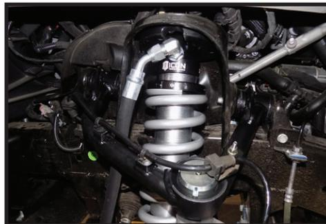
**16.** Secure the harness to the UCA with the supplied M6 hardware and push the clips into the arm. Install dust cover with the supplied 3M tape. [FIGURE 16 & 17]
