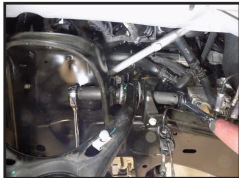
**12.** Now the ICON Tubular UCA can be prepped and assembled. You will want to apply a high quality Moly grease to the inner and outer diameter of each bushing before installing them into the UCA. Once installed with the sleeve and load ring, Apply a layer of grease to the outer surface that will contact the frame mount pockets. Install the supplied 90° grease zerks so that the zerk faces out when installed. [FIGURE 13]
