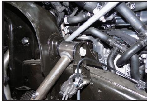
**14.** Slip the coilover into place and secure with OEM hardware if using the OEM coilover or refer to ICON Coilover instructions for specific hardware.
