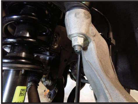
**7.** Now support the knuckle with a strap to the frame to keep it from fall away and pulling apart the CV axle. Then remove the nut from the upper ball joint. The knuckle should rotate out of the way to easier access the coilover.
