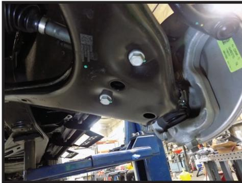
**9.** Remove the 3 18mm nuts from the top of the coilover. There is a wire loom clip on one of the factory studs, use a screw driver or small pry bar to remove it. For easier access, half of the fender liner can be removed and folded out of the way using a T15 torx and plastic clip removal tool. [FIGURE 6 - 9]
