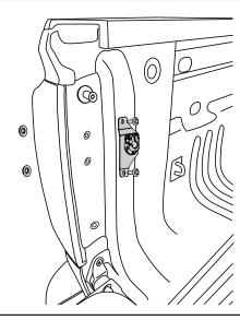
Place Mounting Bracket aligned with top hole. Allow bracket to hang vertically. Mark (Center Punch) location of lower hole using the bracket slot as a template. Remove bracket. Drill hole with 1/8" drill bit then drill out hole with 21/64" drill bit. Use file to remove burrs. Apply primer to edge of hole. Allow primer to dry.
