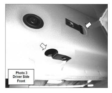
**Step 3** Attach one of the brackets to the rocker panel using (2) M8 SEMS bolt, **(Photo 4 & 5).** Leave the bolts loose for final adjustment.
