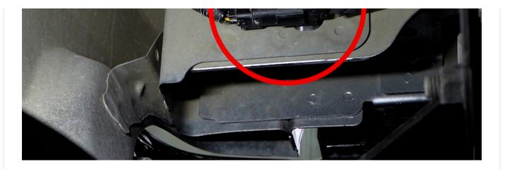
Next, install the provided harness inline with the factory connectors making sure to push the locking tab back into the lock position.
