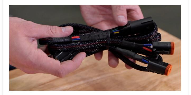
If you're installing the C1R LED Pods that include the additional fourth brake light and optional safety strobe feature, use the harness with the external driver.
