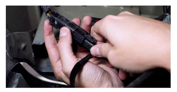
Route the rest of the harness up over the frame and spare tire to the driver's side. Then, repeat these steps to connect the other end of the harness inline with the driver's side tail light connector.
