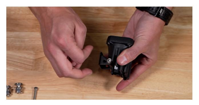
Next, feed the carriage bolt through the oval hole in the U-bracket and reverse brackets. Secure it hand-tight with the washer, lock washer, and nut.
