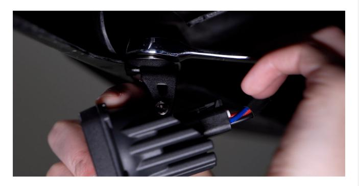
Tilt the pod up or down, then secure it in place with a 5/32 allen wrench and 3/8" wrench.
