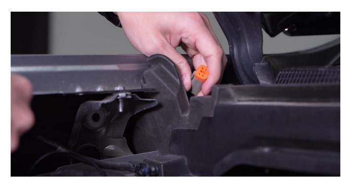
For the driver's side, we'll route the other DT connector across the engine bay away from any hot or moving parts, through the fender bracing, up under the hood, and into the back of our pods.
