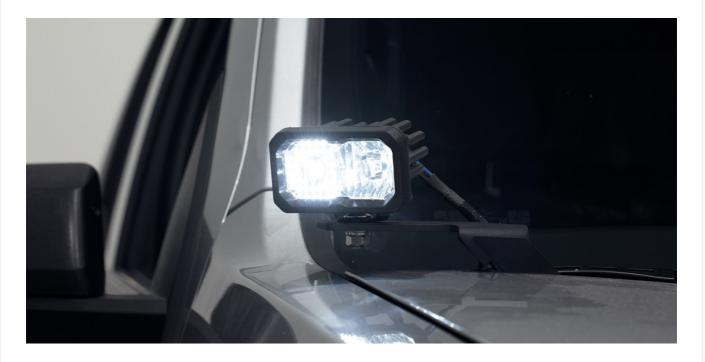
Secure any loose wiring away from hot or moving parts using the zip ties included with our kit.
