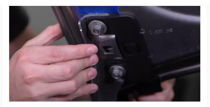
Step 4 - Secure Bracket and Hood Hinge
