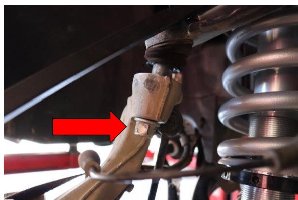
Step 18. Install and tighten the 18mm ball joint nut to manufacturer specification.
