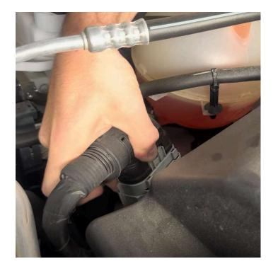
Disconnect the MAF by unlocking the tab and then depressing the lever as you pull it off.
