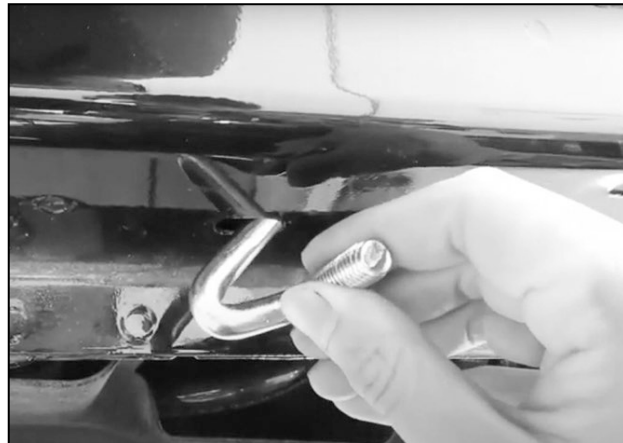
(Fig 4) Insert the tail on the Spiral Bolt into the slot, keeping the threads pointed outwards
