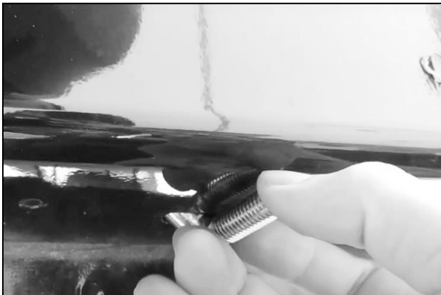
(Fig 5) Insert the bend on the tail into the slot, keeping the threads pointed outwards
