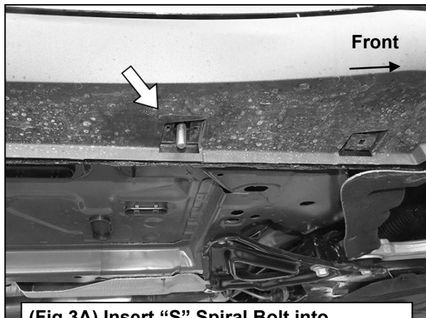
(Fig 3A) Insert “S” Spiral Bolt into opening after removing clip (arrow)
