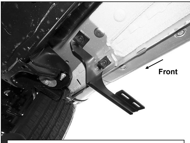
(Fig 3) Passenger/Right Front Bracket installed
