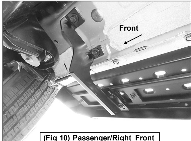
(Fig 10) Passenger/Right Front Running Board installed
