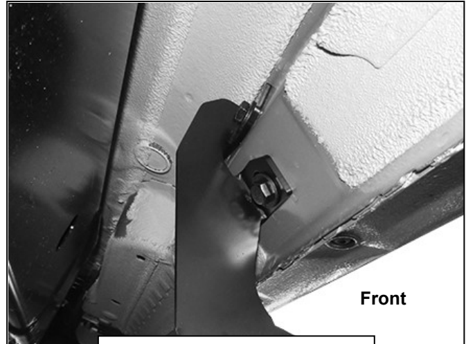
(Fig 6) Front Bracket installed
