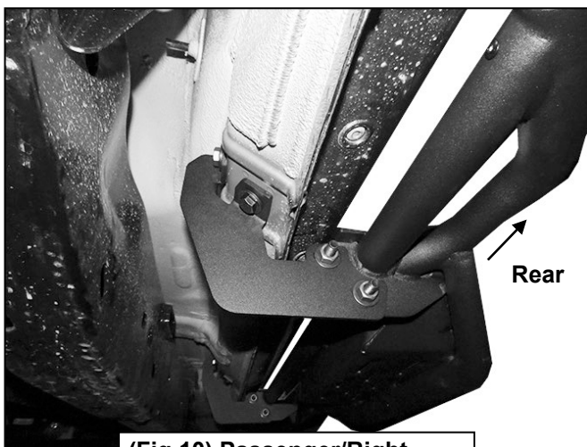
(Fig 10) Passenger/Right Rear Running Board installed
