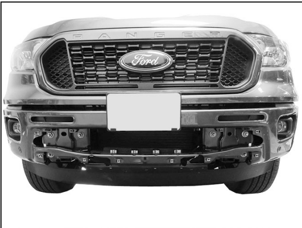
(Fig 3) Center plastic cover removed
