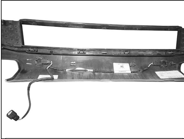
(Fig 15) Models with sensors, remove sensors and harness from plastic panel
