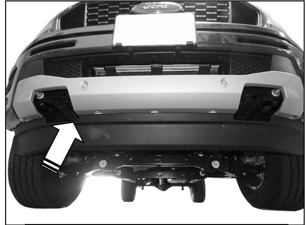
(Fig 2) Remove the center plastic cover from the factory bumper (arrow)
