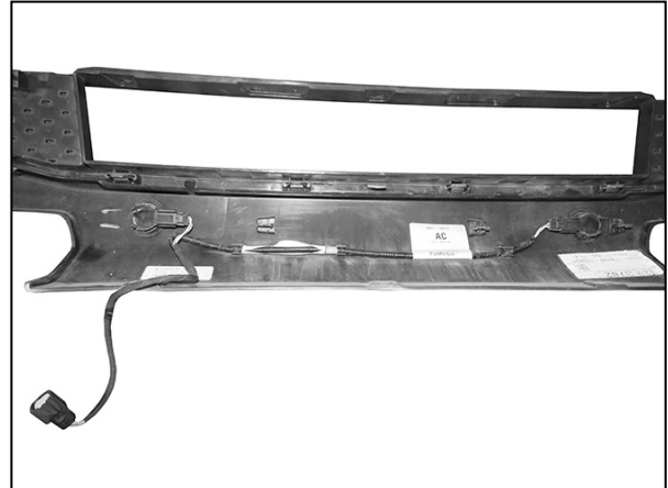
(Fig 19) Models with sensors, remove sensors and harness from plastic panel
