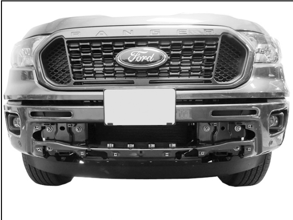
(Fig 3) Center plastic cover removed
