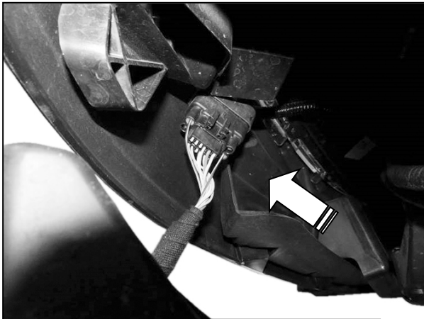
(Fig 5) Pull the bumper out slightly and unplug the outer wire harness
