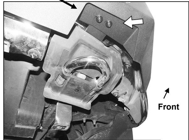
(Fig 28) Attach bottom of Bumper to Support Bracket
