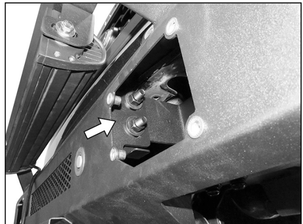
(Fig 26) Driver/left side of Bumper attached to Double Bolt Plate
