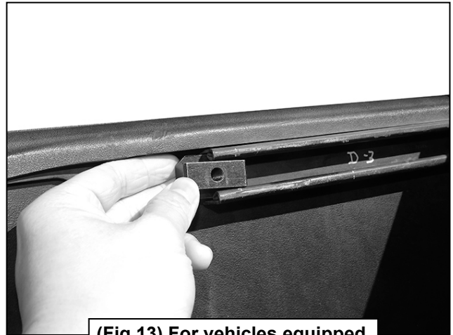
(Fig 13) For vehicles equipped with a bed rail, insert (6) Block Nuts into each side of the bed
