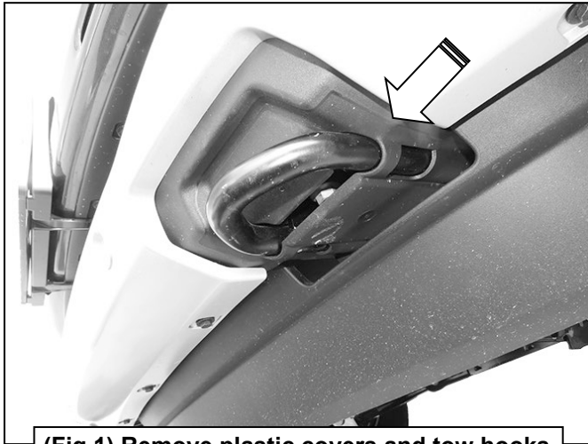
(Fig 1) Remove plastic covers and tow hooks
