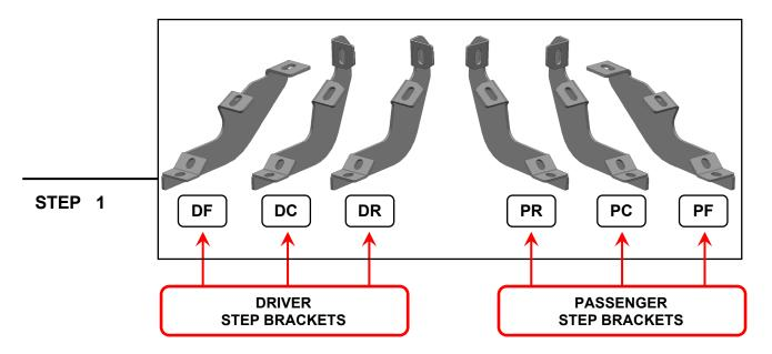
Please identify each mounting bracket using the engraved location identifier. Notice: The center bracket and rear bracket are interchangeable.
