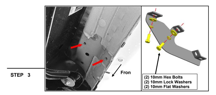
Start installation toward the front of the Passenger/Right side of the vehicle.
