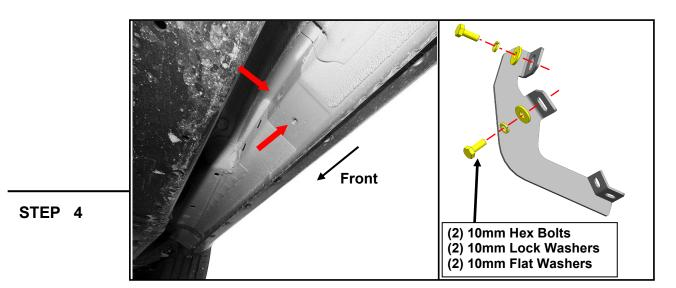
Remove the plastic plugs. Loosely fit the (1) Passenger Center bracket to the vehicle threaded body hole using (2) M10 x 25mm bolts, (2) M10 lock washers, and (2) M10 flat washers. Do not fully tighten to allow for later adjustments. Repeat this step for the Passenger Rear bracket.
