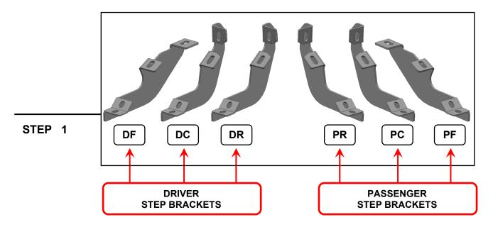
Please identify each mounting bracket using the engraved location identifier. Notice: The center bracket and rear bracket are interchangeable.
