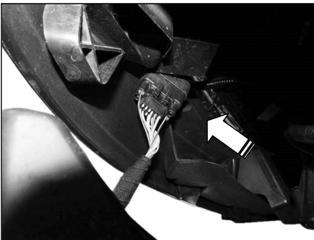
(Fig 7) Pull the bumper out slightly and unplug the outer wire harness
