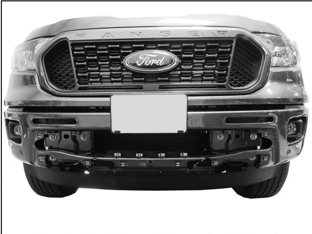
(Fig 5) Center plastic cover removed
