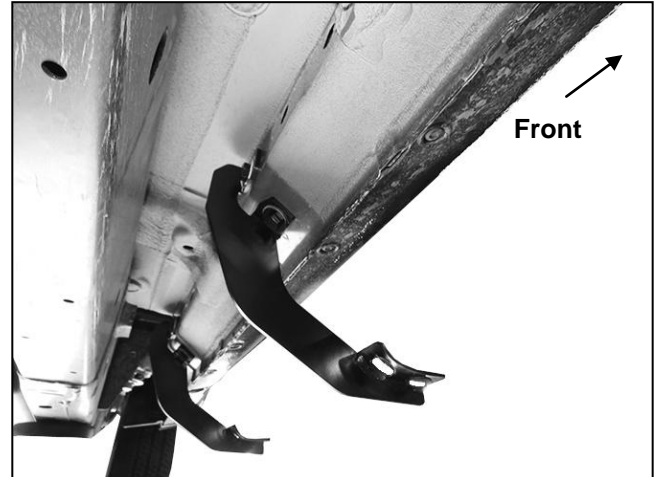
(Fig 6) Driver/Left Center Mounting Bracket installed
