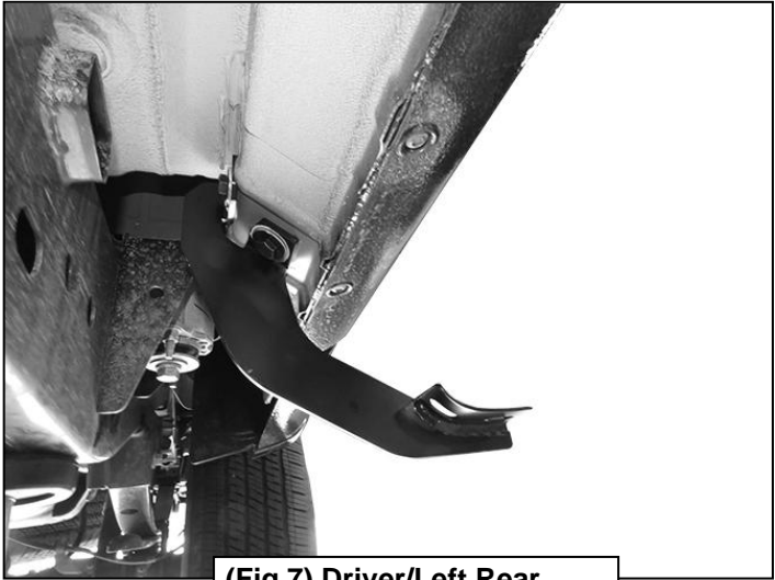
(Fig 7) Driver/Left Rear Mounting Bracket installed
