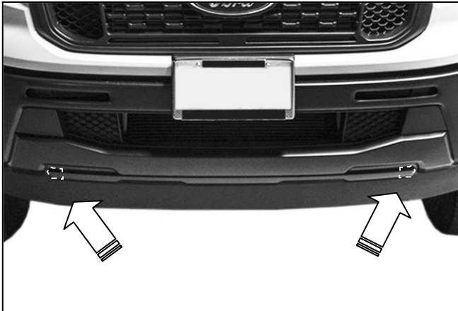
(Fig 5) Models without tow hooks, cut openings in lower plastic cover to clear Brackets
