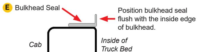
**NOTE:** Position bulkhead seal tight against rail endplug seal and bedcap.
