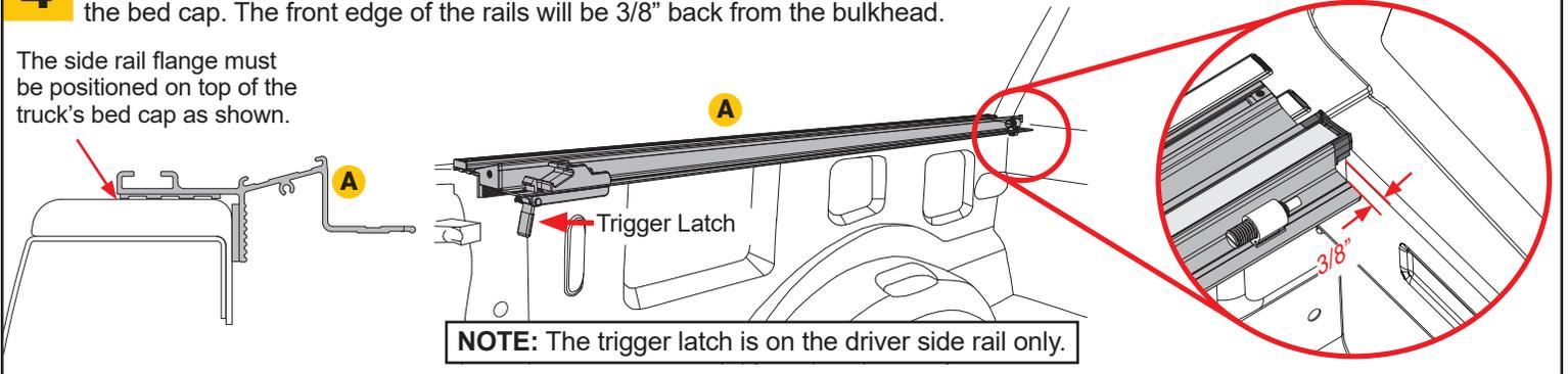
**NOTE:** The trigger latch is on the driver side rail only.
