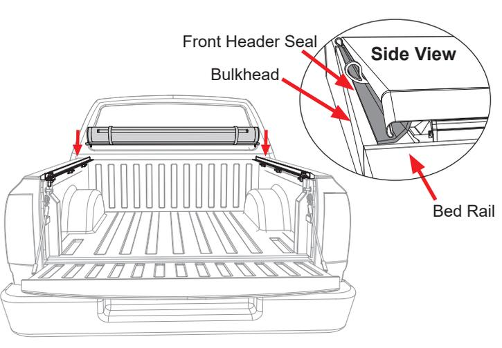
**10** To connect the cover assembly (C) to the side rails (A and B), slide the right and left header guides into the locked position. A clicking sound will indicate a secure attachment.
