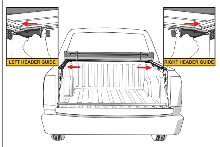
**11** Disengage the retainer hooks from the retainer loops and unroll the cover towards the tailgate.
