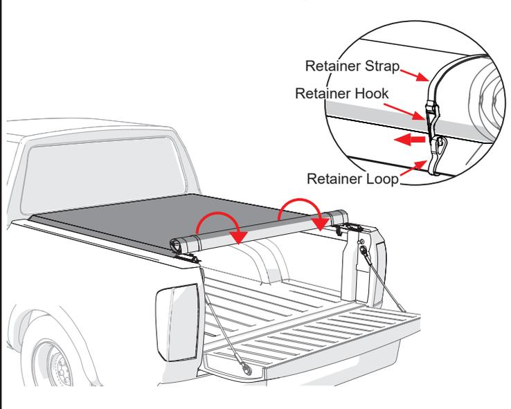
**12** Place the rear header into the header stops which are located on both side rails. Rotate the rear header downwards until you feel the cover latch in place. A clicking sound will indicate a correctly installed cover.
