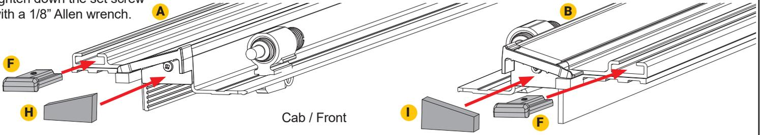
**4** Position the driver side rail (A) to the inside of the truck's bed rail, making sure the flange of the driver side rail fits on top of the bed cap. The front edge of the rails will be 3/8" back from the bulkhead.
