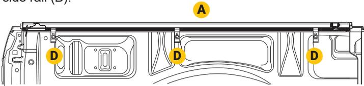
**NOTE:** The use of spring clamps to hold the side rail in place can assist during the installation process.
