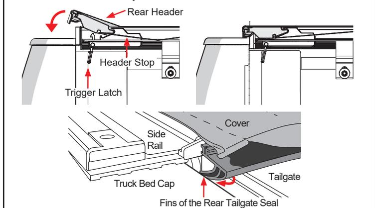
**NOTE:** When you close the tailgate, it pushes the fins toward the inside of the bed with the rest of the seal partially on top of the tailgate.
