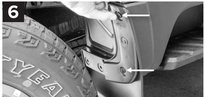
In the top and bottom holes from step 3, install (2) two supplied plastic fasteners. First insert the body, then press the center until flush to lock them in place.
