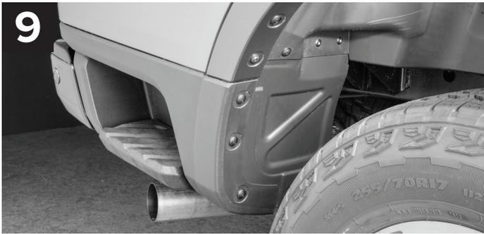
Install the passenger side MudFlap marked "RH," repeating Steps 3-8.
