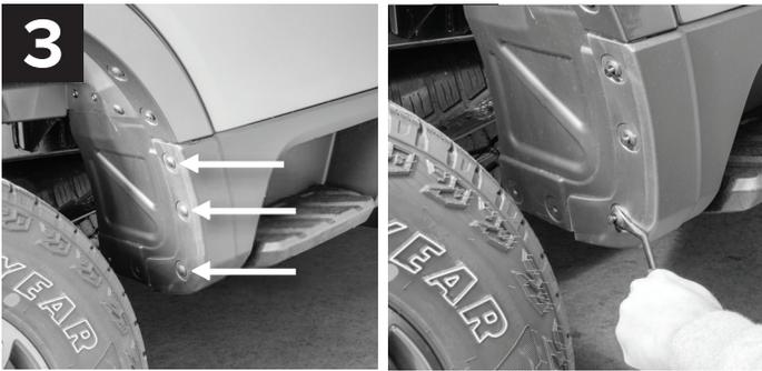
Locate the (3) three plastic fasteners as indicated. Remove by gently unscrewing the centers and then prying out the body. Sometimes it is necessary to use a sharp tool to pry the centers out. These will not be reused.
