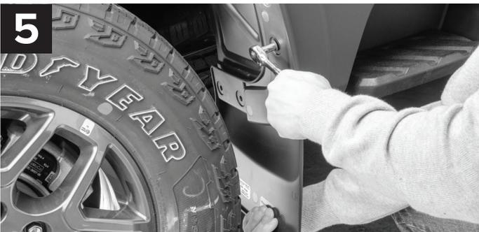
Using the MudFlap marked "LH," place it up to the fender and align with the corresponding holes in the vehicle. Loosely install (1) one supplied hex head screw in the hole where the U-Clip was installed.
