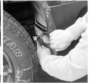
While firmly pressing the MudFlap to seat it properly on the fender, fully tighten the hex head screw and (2) two Phillips head screws.
