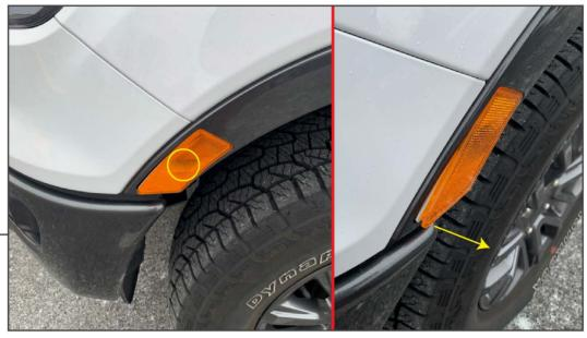
Reach in between the marker light and the inner fender liner. Reach half way up the backside of the light and press up on the tab, while pulling out the bottom corner of the light.
