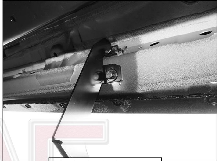
(Fig 6) Driver/Left Center Mounting Bracket installed
