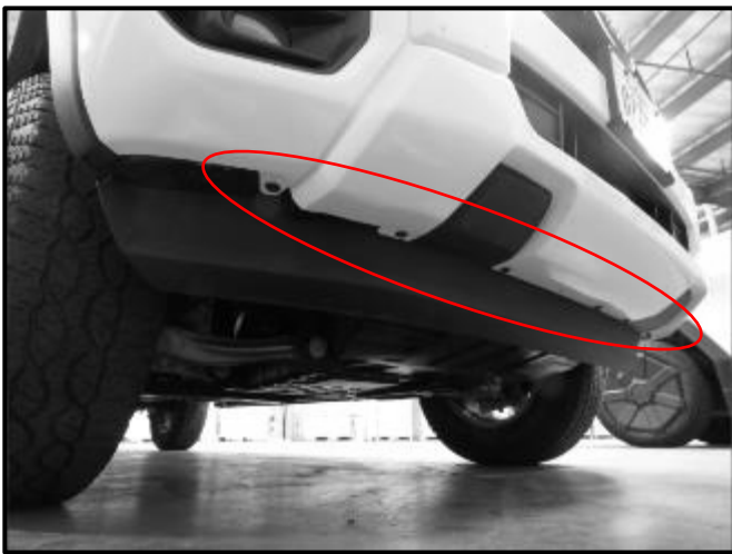
(Fig 1) Remove the Air Dam by removing the bolts along the bottom edge of the Front Fascia.
