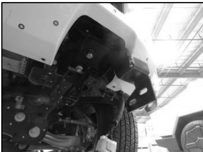
(Fig 5) The Mounting Bracket is now installed.
