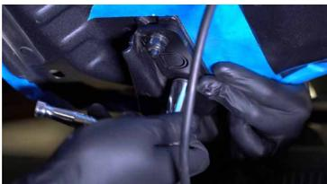
5. Secure the bracket and hood hinge by tightening the factory bolts, ensuring the hood hinge lines up with the tape.
