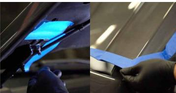
2. Mark the location of the hood hinges with tape and tape the edges of the hood to prevent scratching.
