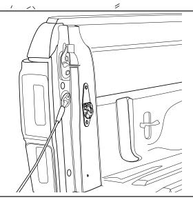
Tighten fasteners. Make sure pivot opening in bracket opens towards the rear of the vehicle.
