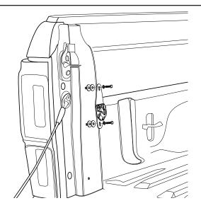
Install Pivot Brackets to upper two threaded holes on D-Pillar. Each bolt location will take two plastic spacers (4 total per bracket, as shown) under the bracket to properly space brackets.
