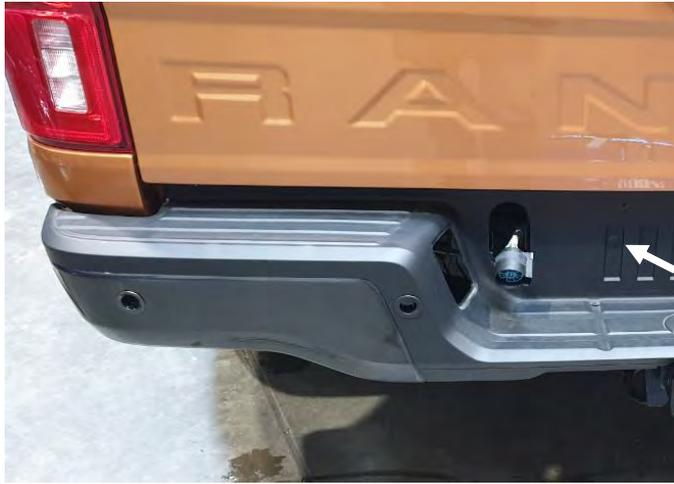
7. Unclip the parking sensors from the OE housings by unclipping them from behind the bumper.
