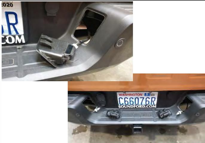
2. Unclip the number plate lights from behind the bumper and remove.
