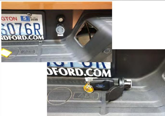
4. Using the vehicle key, remove the locking plug for the spare wheel access. Set aside for use in the ARB rear bar.
