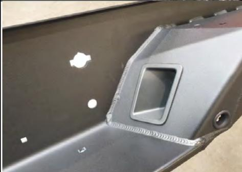
37. Re-fit the rear number plate globe and then clip in the OE number plate light assembly as shown. Ensure that both tabs are clipped properly on the bracket.
