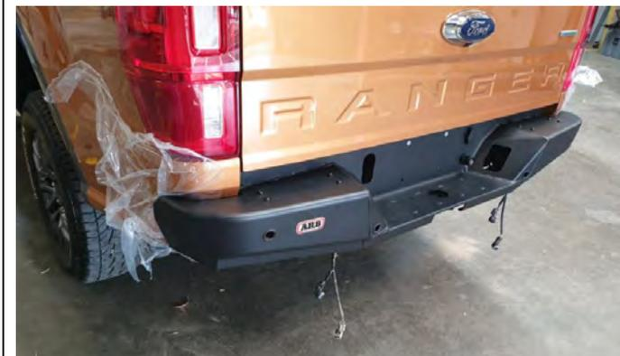
27. Lift the rear bar carefully on to the OE tow bar as shown. Be careful not to damage the rear bar or the vehicle.
