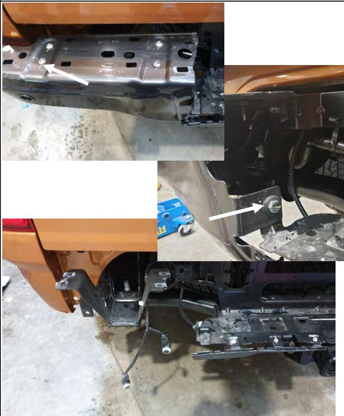
10. Remove the 4xM8 Torx bolts on the top of each steel bumper end.
