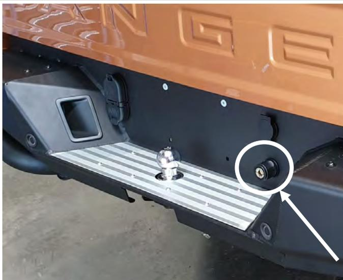
38. Fit the number plate using 4 plastic gromets and black screws.
