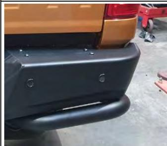
34. Re-adjust the lower protection rails so that they are parallel to both the vehicle body and the rear bar wing.
