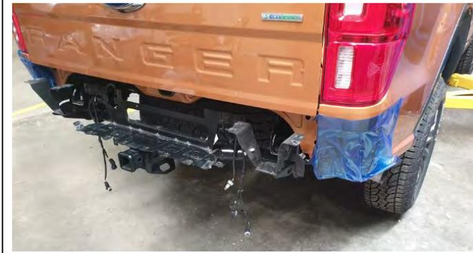
***Use a low tack film or similar to protect the rear quarter panels of the vehicle while fitting the rear bar.***
