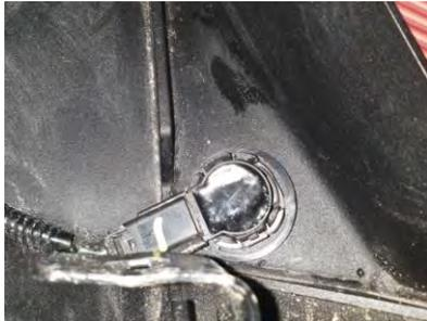
36. Clip the 4x parking sensors into the housings, ensuring the rubber sleeves are still on the sensors and that they don't catch/pinch when sliding into the housing.
