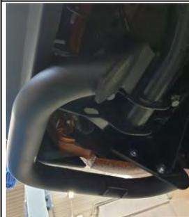
31. Adjust the rear bar so that it has an even gap on both wing tips to the vehicle body. Adjust the lower protection rails so that they are parallel to both the vehicle body and the rear bar wing.
