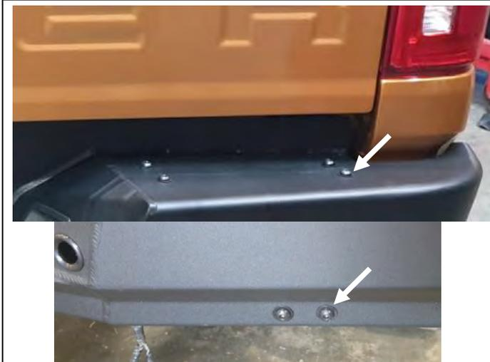
28. Use 8x black M8x25 button head bolts and black M8 flat washers on the top of the bar (4 bolts and washers per side) to affix the bar to the upper tow bar brackets. Leave loose at this stage.
