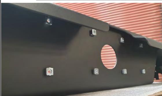
22. Loosen the M16 OE tow bar retaining bolts on one side. (The light-duty tow bar has 2 bolts each side. The heavy-duty tow bar has 3 bolts each side).
