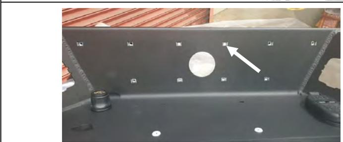
21. Fit 10x M6 cage nuts to the under-side of bar for the treadplate.
