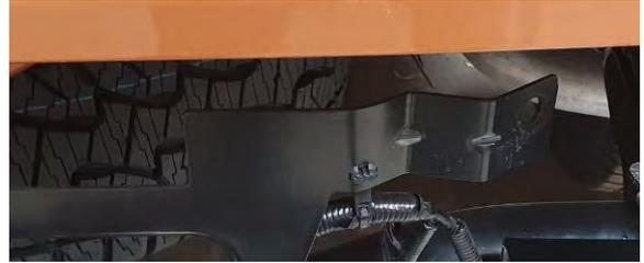
16. Bend the lower tabs down by 90deg as shown:
