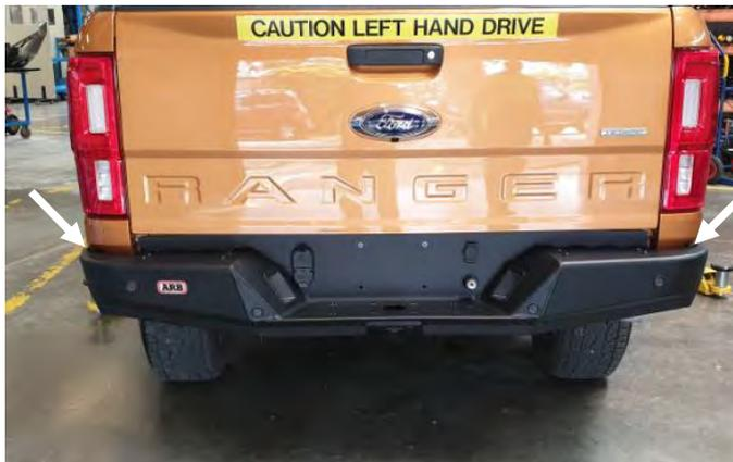
29. If only fitting the rear bar, adjust the bar so that it sits with an even gap at both wing tips. Tighten the 12x M8 bolts to the specified torque. Tighten the main tow bar M16 bolts to the specified torque. Skip to step 36.
