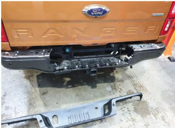
9. Unclip the upper plastic trim from the steel bumper assembly.
