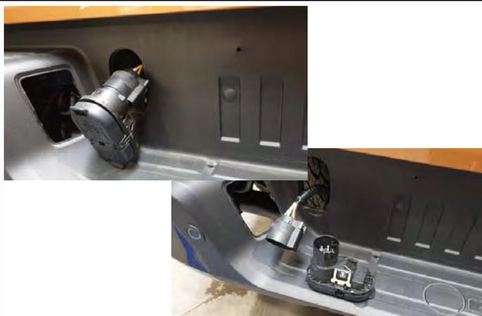
5. Unclip the smart trailer plug from behind. (Heavy duty tow pack models only).
