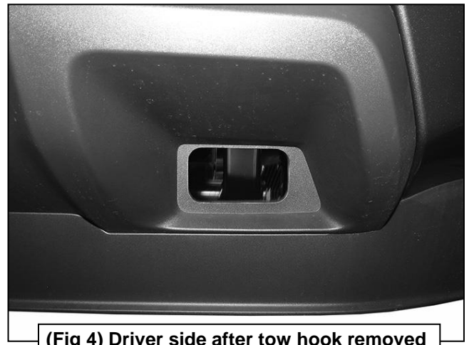
(Fig 4) Driver side after tow hook removed
