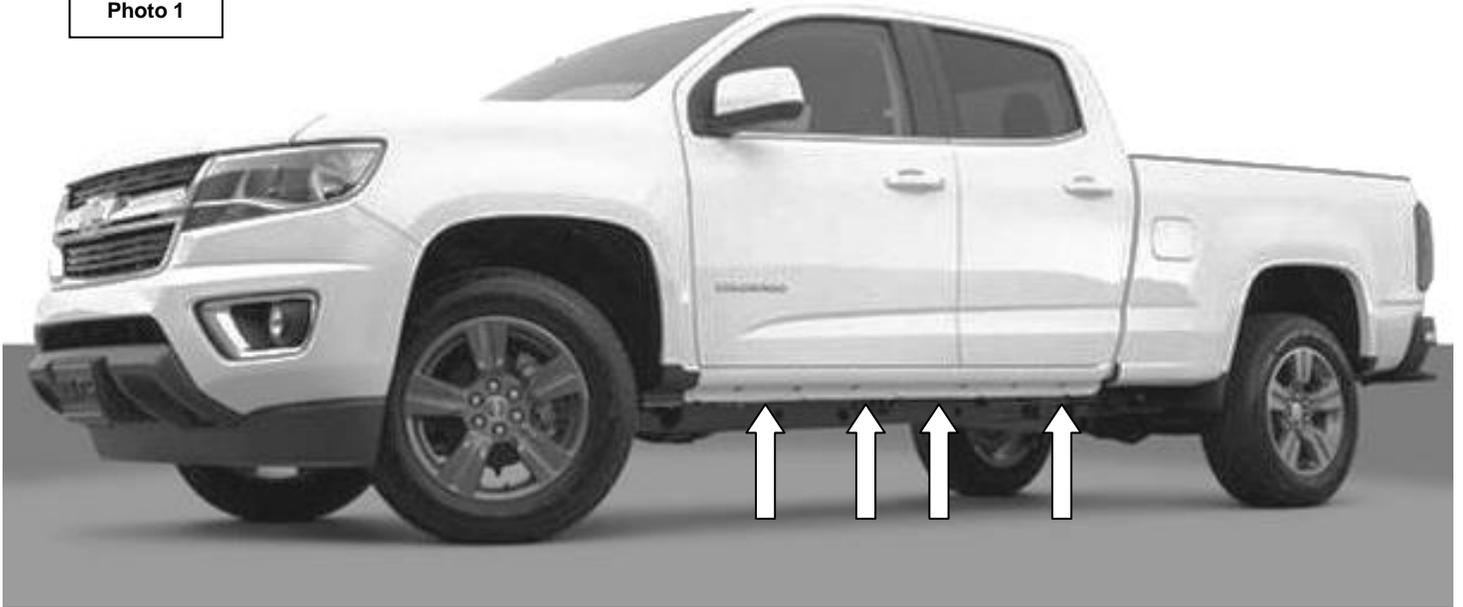
**Step-1** Begin the installation on the driver side. Starting at the front of the vehicle, locate and remove the plastic plugs in the back side and bottom of rocker panel to expose the holes used for placement of the M8 Clip- Nuts, (Photo 2).
