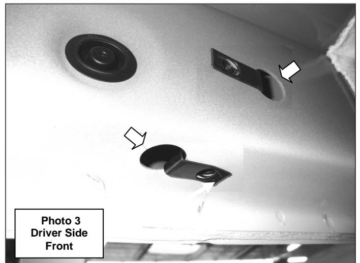
**Step-3** Attach one of the brackets to the rocker panel using (2) M8 hex bolts, (Photo 4 & 5). Leave the bolts loose for final adjustment.
