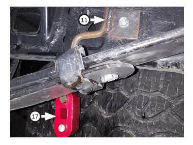
12. Route **left overaxle (5)** and **right tailpipes (4)** over axle then connect them to muffler. Insert wire hangers into isolators then tighten clamps just enough to allow for adjustment.
