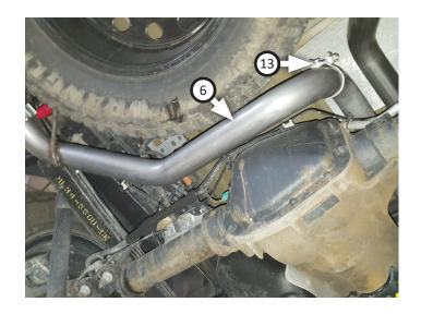
14. Place (x2) clamps (13) onto side exit pipe (7) then connect them to tailpipes and tighten clamps just enough to allow for later adjustment.
