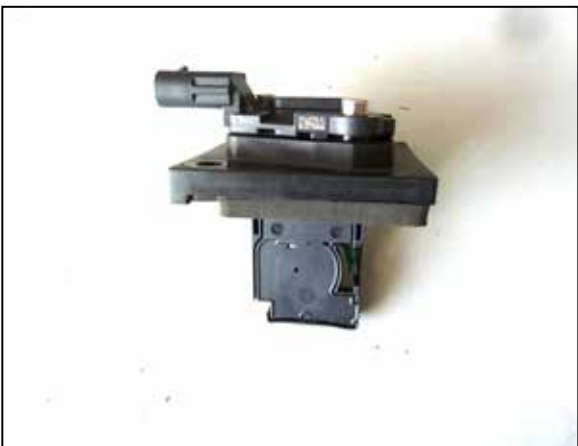
16. Remove the MAF sensor using T20 torx from the air box. Install to the MAF adaptor. Secure using provided hardware and attach gasket to the bottom of the adaptor.
