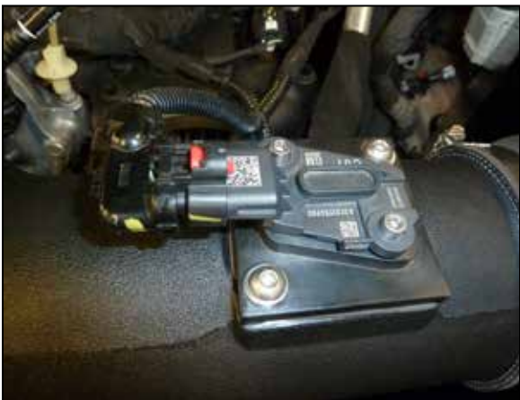
22. Reconnect the MAF sensor harness. Reconnect the vacuum line to the fitting on the K&N intake tube.
