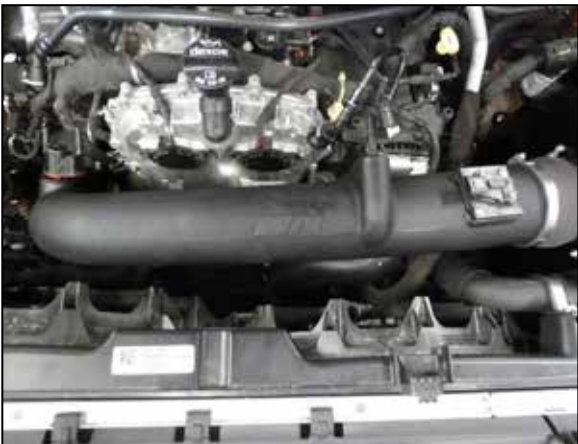
20. Install the K&N intake tube into vehicle and position. Tighten clamps.
