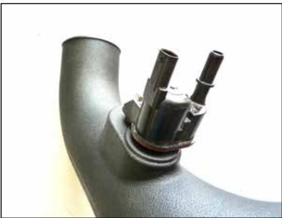
19. Loosen the 10mm bolt holding in the CCV solenoid and remove from OEM intake tube. Install to the new K&N intake tube.
