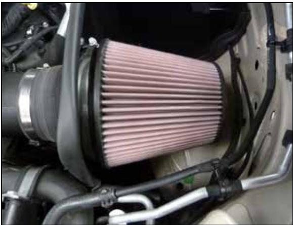
23. Install the K&N filter to the adaptor. Secure and tighten.
