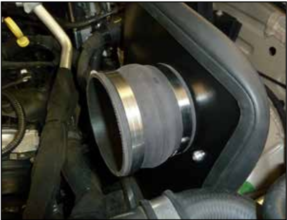
15. Install the step hose with clamps to the turbo. Install the hump hose with clamps to the filter adaptor.
