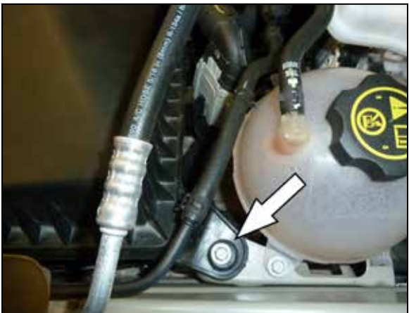
8. Remove the bolt holding in the air box. Pull any harness lines attached to the air box, and pull back ECU relay harness away from air box using pliers or flathead screw driver. Carefully remove the air box out of the vehicle. NOTE: K&N Engineering, Inc., recommends that customers do not discard factory air intake.
