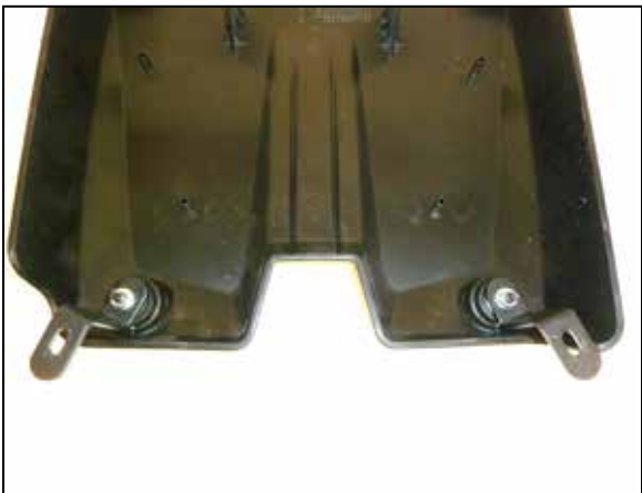
24. Install the Z brackets to the engine cover like image shown. Use OEM bolts and secure using provided serrated nuts.
