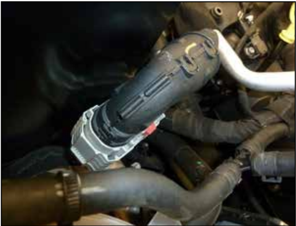
14. Attach the ECU relay harness to the slot cut out on the back of the heatshield.
