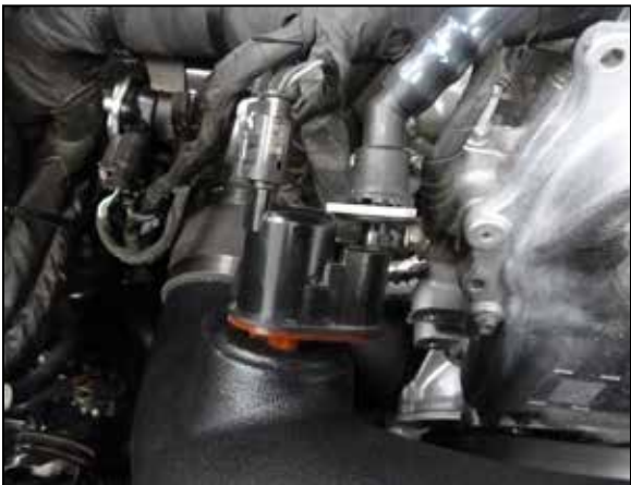
21. Reconnect the CCV line and harness to the solenoid.
