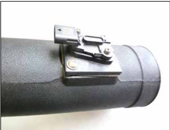
17. Secure the MAF adaptor assembly to the K&N intake tube using provided hardware like image shown. Note: Make sure the MAF sensor is going in correct direction.
