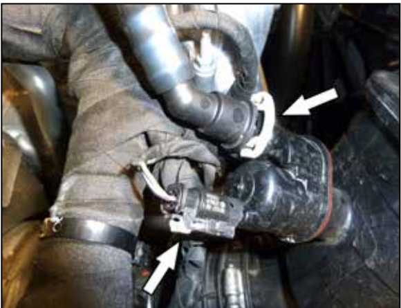
4. Locate the CCV solenoid on the back of the intake tube and depress the CCV locking tab and disconnect the harness.
