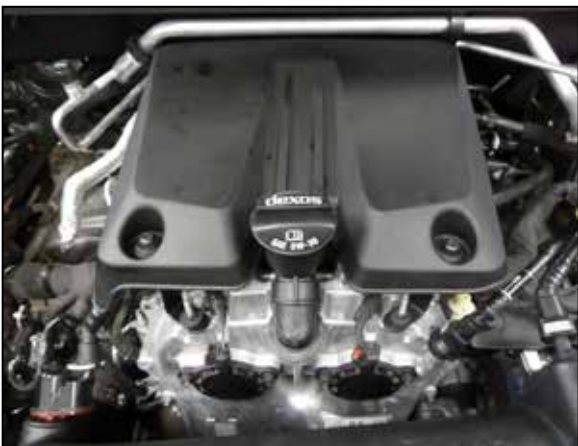
25. Install the engine cover and secure the Z brackets to the OEM intake tube locations using OEM nuts. Secure and tighten.
