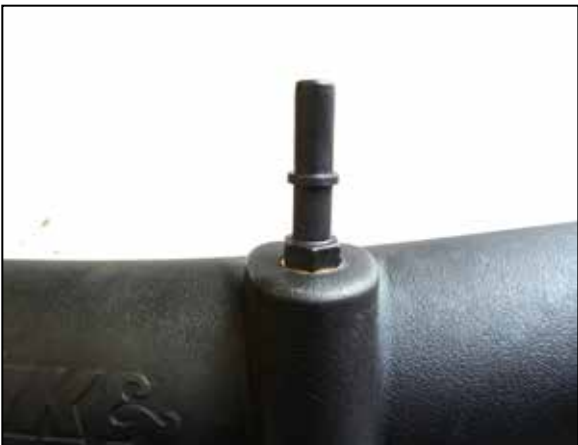
18. Install the quick connect to the threaded insert on the K&N intake tube. Secure and tighten.
