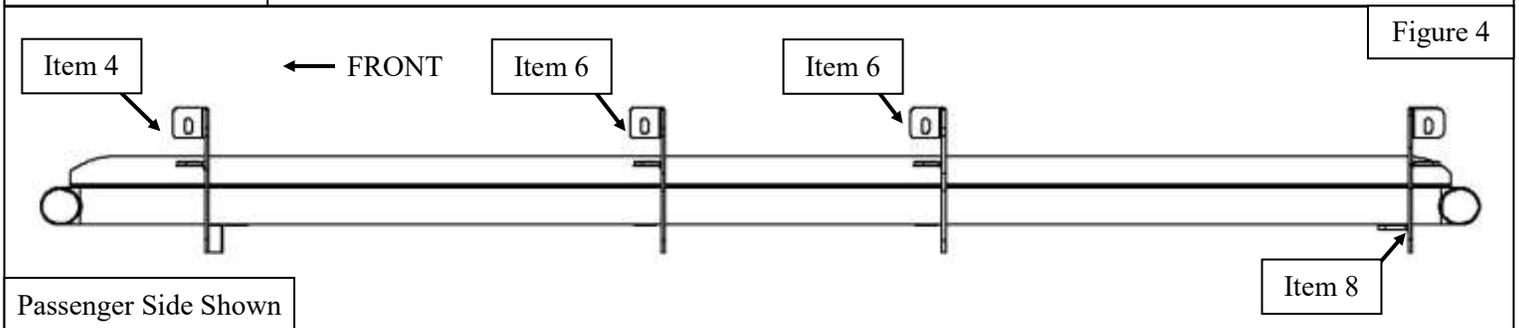
5. Use the supplied M10 hardware to mount and secure the Outlaw Running Board (Item 1) to the previously installed mounting brackets. See **Figures 5 & 6** for reference.
