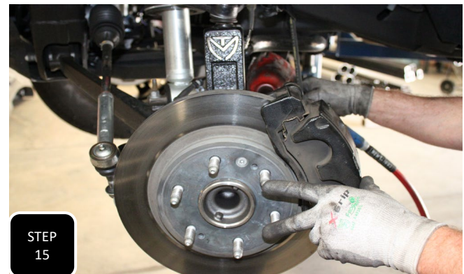
Step 15 Remove the clip that attaches the soft brake line to the frame and pull the hard line through the bracket to gain slack in the line. Next, install the brake caliper using the factory bolts and tighten to factory specs.
