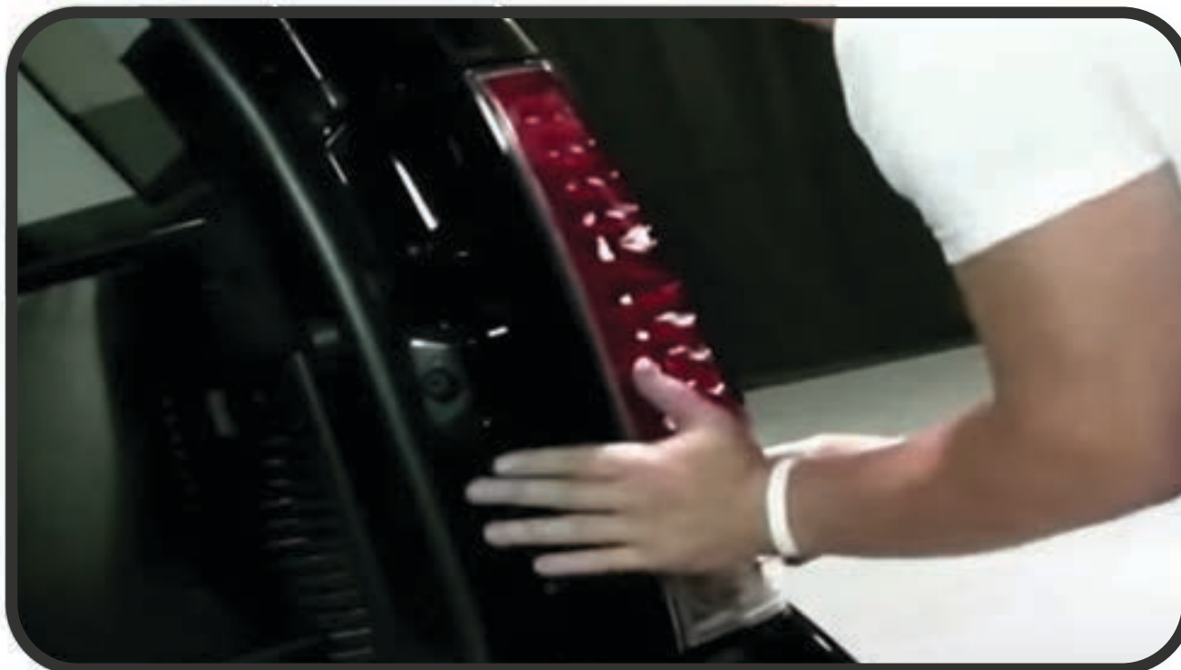
STEP 7: SEAT THE SPYDER TAIL LIGHT AND REINSTALL THE (2) PHILLIPS SCREWS TO SECURE IT IN PLACE
