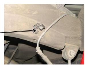
Remove the ride height sensor bracket.
