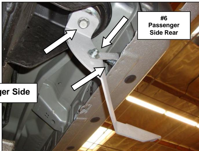
**Step-7** Place the passenger side running board on top of the mounting brackets. Position (3) of the U-brackets inside the running board body, and align the U-brackets with the holes in the mounting brackets. Attach the running board to each mounting bracket using the U-bracket, (2) 5/16" hex head bolts, (2) 5/16" flat washers and (2) 5/16" lock washers, (Photo 7).
