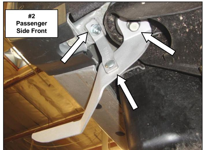
**Step-3** Remove the passenger side middle body mount bolt. Keep all existing bushing in place, and attach the passenger side middle bracket to the vehicle using the factory body mount bolt, (Photo 3 & 4). Leave the body mount bolt loose for final adjustment.
