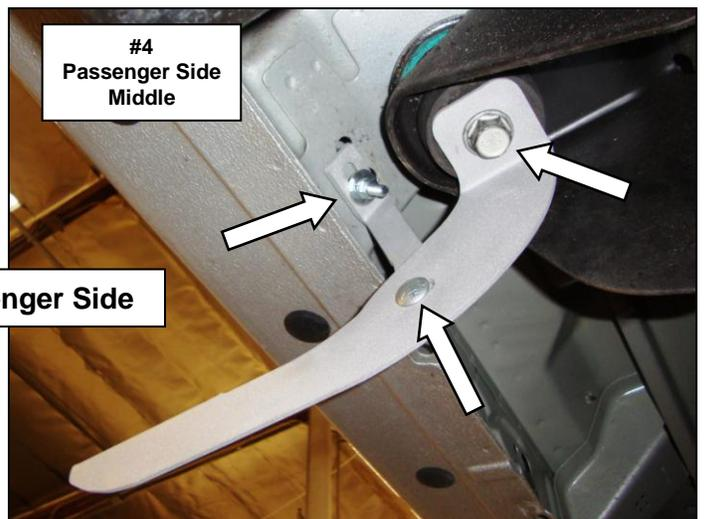
**Step-5** Remove the passenger side rear body mount bolt. Keep all existing washer and bushing in place, and attach the passenger side rear bracket to the vehicle using the factory body mount bolt and supplied 1/2" flat washer, (Photo 5 & 6). Leave the body mount bolt loose for final adjustment.
