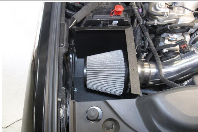
20. Install the provided HPS performance air filter.
