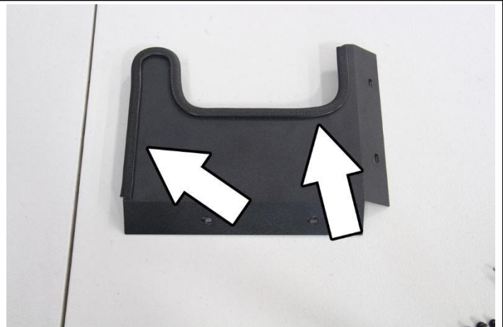
21. Insert the provide edge trim onto the heat shield lid shown in the indicated areas shown above.
