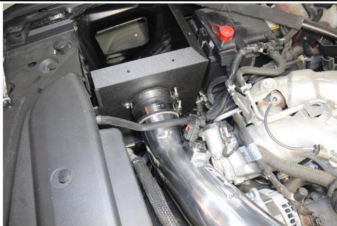
18. Slide and secure the reducer coupler above the velocity stack and the intake pipe.
