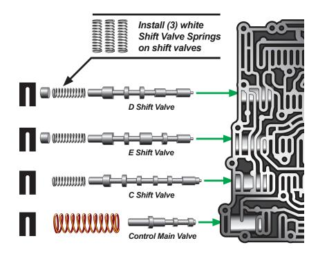
Install the three PPE white springs on to the D, E and C Shift Valves.
