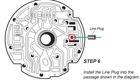
Stake with a chisel at the top of the bore to keep the Line Plug from moving out of position.
