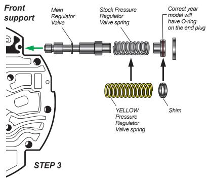
Install new YELLOW Pressure Regulator Valve spring.
